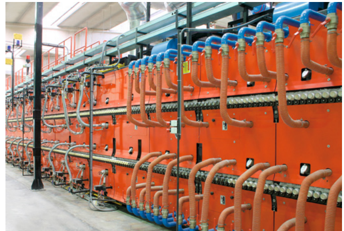
Roller hearth kiln in the ceramics industry
