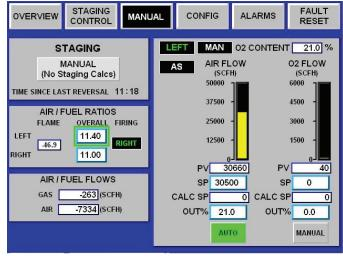
Figure 4.6. Manual Staging Control Screen
