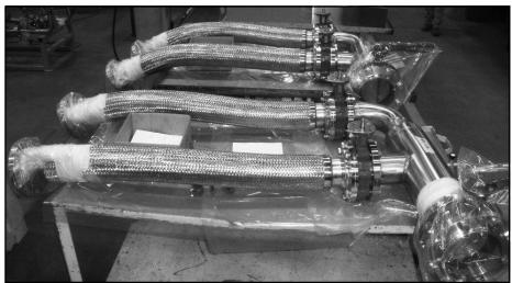
Figure 3.6. Supply Header with Hoses for Endport Furnace (Note: Two injector supply headers shown)
