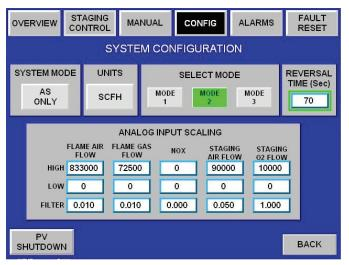
Figure 4.13. System Configuration
