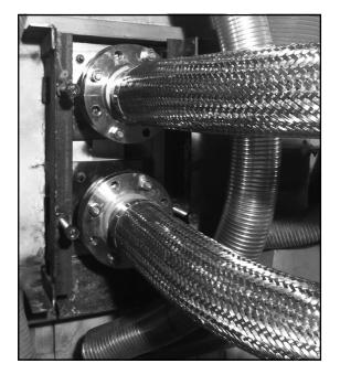
Figure 3.3. Injector for Endport Furnace (Note: Two injectors shown stacked)
