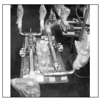
Figure 3.1. Metering Spool / Upcomers (Note: Two injector metering spools shown)
