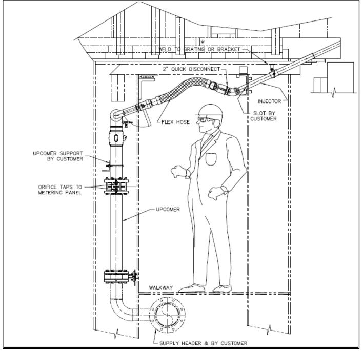
Figure 3.8. SideFired Injector Layout (Section through port alley between furnace and regenerator)
