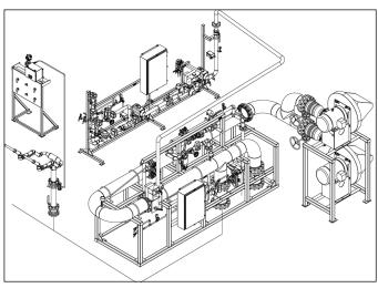
Figure 1.1. Oxygen Enriched Air System
