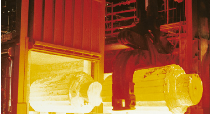
Metallurgical industry: forging furnace
