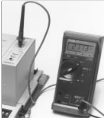
Voltmeter hook-up to a Bi-Flame
