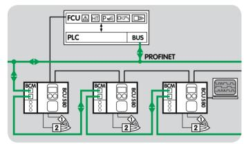
The basic function of Profinet is the exchange of process and required data between an IO controller (e.g. PLC) and several distributed IO devices (e.g. BCU/FCU).
