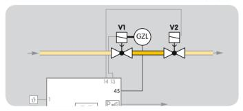
By checking the closed position using the proof of closure function, the BCU complies with the requirements of NFPA 85 (Boiler and Combustion Systems Hazards Code) and NFPA 86 (Standard for Ovens and Furnaces).
