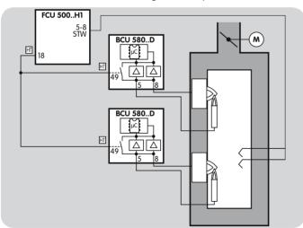
When the HT input is activated (terminal 49), the burner control unit reverts to High temperature mode, i.e.: the BCU operates without evaluation of the flame signal. The safety function of the device-internal flame control system is deactivated.
