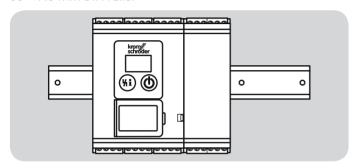
If the DIN rail is aligned vertically, end clamps are required (e.g. Clipfix 35 by Phoenix Contact) to prevent the BCU from slipping.
