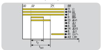
If no flame is formed during the start-up so that at the end of the safety time  $t_{SA1}$  no flame signal is detected, this will result in a BCU safety shut-down with subsequent fault lock-out. The fault message  $\square$ 4 will flash in the BCU display depending on the burner operating mode.
