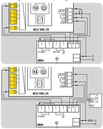
The RBW actuator reports that it has reached the position for maximum capacity via a signal to terminal 51. The actuator
