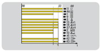
Parameter 43 = 0: Off. No low fire over-run is performed. The gas circuit is closed immediately owing to a quick closing gas valve in the case of On/Off control. The air circuit is closed more slowly. The air flowing in during this time increases the  $O_2$  content in the combustion chamber.
