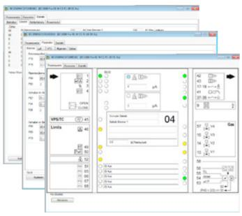
In addition to the engineering tool BCSoft, an opto-adapter or Bluetooth adapter is required to read the device parameters in and out, see also page 106 (BCSoft).
