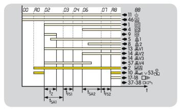
This setting together with parameter 49 = 0, see page 83 (Air actuator can be activated externally on start-up), is required for burners on which the air/gas ratio is controlled by a pneumatic air/gas ratio control system and which need to be started at low-fire rate, e.g. on two-stage-controlled burners, see page 10 (Two-stage-controlled main burner with permanent pilot burner). In this case, activation of the air actuator during burner start via the input at terminal 2 must be prevented.
