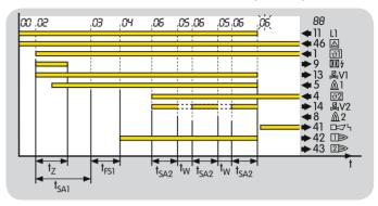
If no flame is formed during the start-up so that at the end of the safety time  $t_{SA2}$  no flame signal is detected, the BCU closes the gas valves and repeats the start-up. Each start-up attempt begins with the parameterized start-up behaviour.
