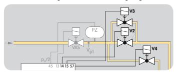
Parameter 52 = 2: V2. The test volume is discharged via the valve connected to terminal 14.
