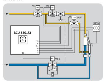
Parameter 42 (Running time) can be used to adjust the behaviour of slow opening and closing air valves so that the system can be set to ignition position before a start-up is initiated. Parameter 41 (Running time selection) must be set to 1 to adjust this behaviour.
