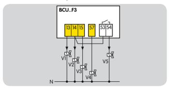
The following application describes a two-stage-controlled burner without a pneumatic air/gas ratio control system. V2 and the air valve are activated simultaneously.
