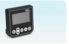
The OCU is an external operator-control unit which can be connected to a control unit of the FCU 500/BCU 500 series. The external operator-control unit OCU may be installed in the door of a control cabinet, for example. Thus, the control cabinet does not need to be opened to read out process values, statistics, flame signal intensities or parameter values, to change settings on the OCU or to control or adjust connected butterfly valves in Manual mode.
