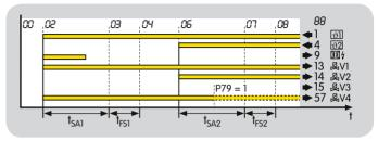
If a burner with a pilot burner is used, this parameter can be used to define whether the pilot burner is shut down 1 second before the end of the second safety time  $t_{SA2}$  or operates continuously.
