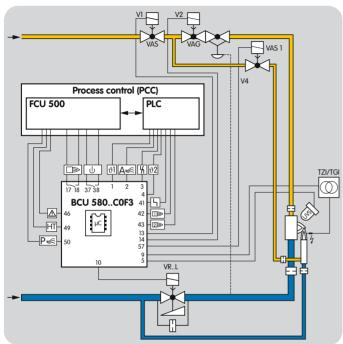
The BCU..F3 activates an air valve for purging, cooling or starting the burner. The required air capacity is released by the air valve.
