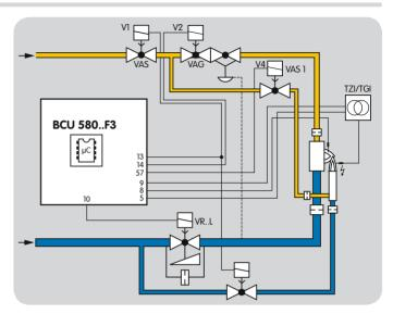
This means that the burner is initially adjusted down to low fire and then switched off completely. Flame control is still operational. It must be ensured that no excess gas occurs.
