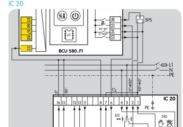
The positions for maximum capacity, ignition capacity and minimum capacity can be set using the actuator. It is checked whether the relevant position has been reached using terminal 52. If the position is not reached within the timeout time of 255 s, the BCU will display fault message  $R_{\Box}$ ,  $R_{\Box}$  or A<sub>1</sub> (maximum, ignition or minimum capacity not reached), see page 47 (Fault signalling).
