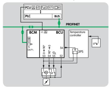
All network components which connect the automation system and the field devices must be certified for Profinet use.
