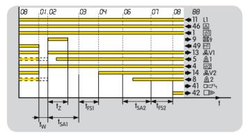
The BCU switches off the burner once the HT input has been disconnected from the electrical power supply and restarts with flame simulation check (recommended in the case of UV control with UVS).
