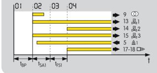
Parameter 78 = 5: burner 1 and two-stage burner 2. In this application, the burner has an additional pilot gas valve V3. The valves are connected to the valve outputs (terminals 13, 14, 15 and 57). Valves V1 and V4 open to start the pilot burner. The burner is started with a limited ignition capacity using gas valve V3. Valve V2 (terminal 14) can be opened with the operating signal (program step 08) in order to operate burner 2 at maximum capacity.
