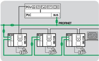
The bus system transfers the control signals from the automation system (PLC) to the BCU/BCM for starting, resetting, controlling the air valve, purging the furnace or for cooling and heating during operation. In the opposite direction, it sends operating status, the level of the flame signal and the current program status.
