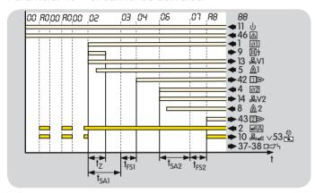
During start-up, the air actuator remains closed. The air actuator cannot be activated externally.
