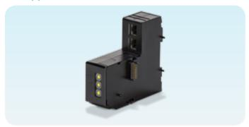
The bus module BCM 500 is used as a communications interface for devices of the BCU/FCU 500 product family for connection to a Profinet network. Networking via Profinet enables the FCU or BCU to be controlled and monitored by an automation system (e.g. PLC).
