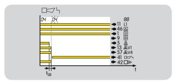
A safety shut-down with subsequent fault lock-out takes place in the event of flame failure during operation.
