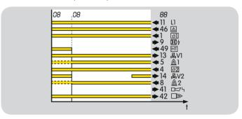
Despite the HT input having been disconnected from the electrical power supply, the burner remains in operation. The BCU performs flame control again (recommended in the case of ionization control or UV control with UVD).
