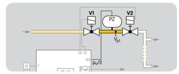
The required measurement time for the tightness test of  $V_{p1}$  can be set using parameter 56. The possible settings are 3 s, 5 to 25 s (in 5 s steps) or 30 to 3600 s (in 10 s steps).
