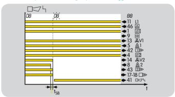
If the flame fails during operation, the output for valve V2 is disconnected within the safety time t<sub>SB</sub>.
