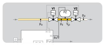
The test period  $t_p$  is calculated from:
