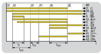
If no flame is formed during the start-up so that at the end of the safety time  $t_{SA1}$  no flame signal is detected, this will result in a BCU safety shut-down with subsequent fault lock-out. The fault message  $\square E$  will flash in the BCU display depending on the burner operating mode.
