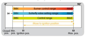
The control system is enabled for operation via the controller enable output (terminal 56). During the controller enable procedure, the actuator can be adjusted infinitely between the positions for maximum and minimum capacity by an external three-point step controller or using bus signals. There is no timeout active in this case.
