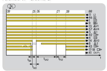
If a flame failure occurs during operation (minimum operating time of 2 s), valve 2 is closed and the operation signalling contact is opened within the safety time during operation  $t_{SB}$ . The burner control unit then attempts to restart burner 2 once. If burner 2 does not function, a safety shut-down with fault lockout occurs. The display blinks and shows the fault message.
