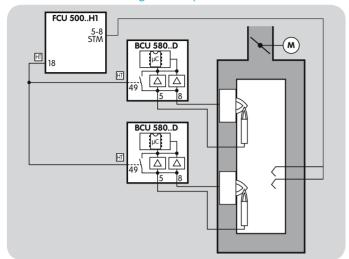
In high temperature systems (temperature > 750 °C), the flame may be controlled indirectly via the temperature.
