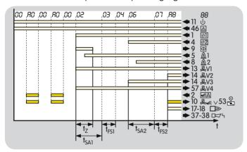
This setting is required in the case of two-stage main burners which are switched ON/OFF via the  $\vartheta 2$  input.
