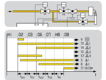
For this application, it must be ensured that the flame proving period (P97) is set to a value  $\geq 2$  s.
