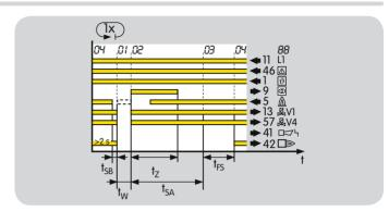
If a flame failure occurs during operation (minimum operating time of 2 s), the valves are closed and the operation signalling contact is opened within the safety time during operation  $t_{SB}$ . The burner control unit then attempts to restart the burner once. If the burner does not function, a safety shut-down with fault lock-out occurs. The display blinks and shows the fault message.
