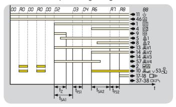
The air actuator opens at the same time as safety time  $t_{\rm SA2}$  begins and the main burner starts.
