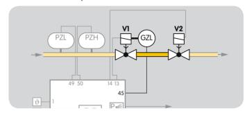
A signal is sent to the BCU via the POC switch on the gas solenoid valve on the inlet side before burner start-up stating that the valve is closed. After burner start-up, the signal must drop out to indicate to the BCU that the valve is open.
