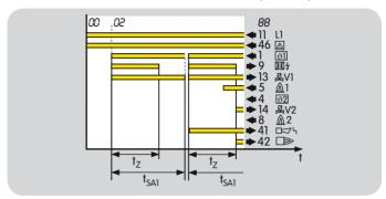
If no flame is formed during the start-up so that at the end of the safety time  $t_{SA1}$  no flame signal is detected, the BCU closes the gas valves and repeats the start-up. Each start-up attempt begins with the parameterized start-up behaviour.
